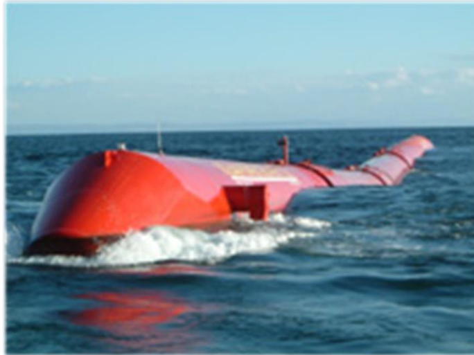
Figure 1.11 - Pelamis type wave power turbine. Water inside the 'tube' flows from one side to the other, thereby rotating small turbines inside the 'tube', which in turn generate electricity.
