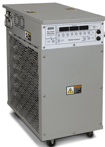
Figure 2.1 - Resistive load banks (ASCO power technologies) of 0.5 MW, with horizontal hot air discharge [20]. The unit shown above is about 1 meter in height.
