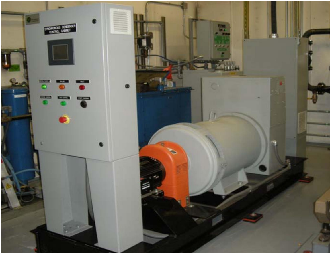
Figure 2.2 - Synchronous condenser, product of Sustainable Power Systems company [21].
