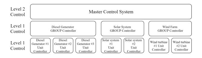
This structure helps the sectionalisation of the system and provides for easier maintenance.
